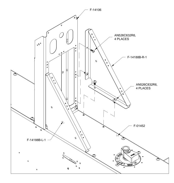
FIGURE 2: BRACKET INSTALLATION
