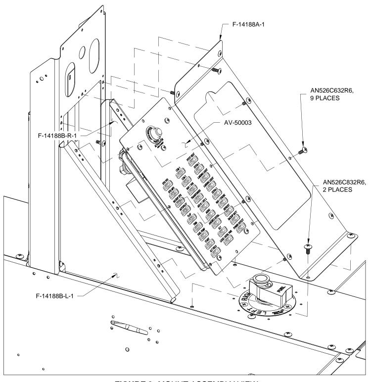
FIGURE 3: MOUNT ASSEMBLY VIEW
