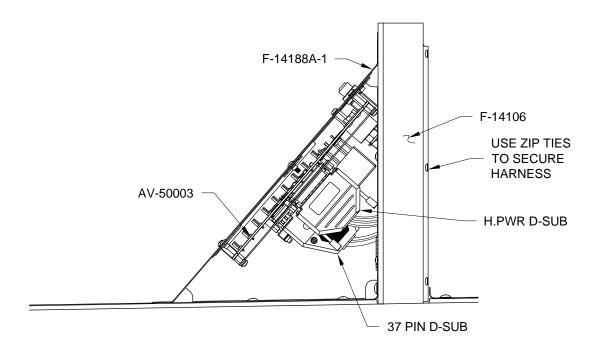
FIGURE 2: WIRE HARNESS ATTACHMENT
