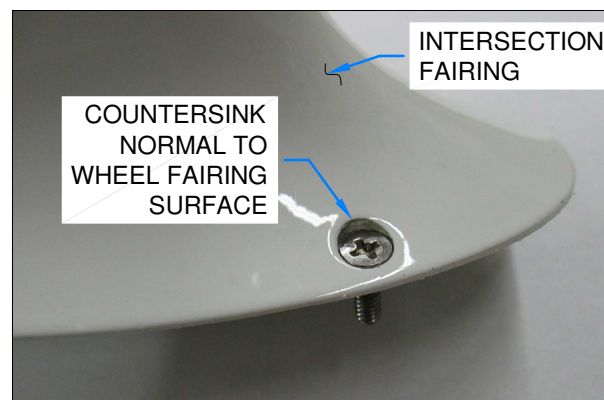
FIGURE 1: COUNTERSUNK INTERSECTION FAIRING SCREW LOCATION
