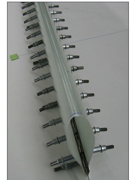
FIGURE 3: DRILLED & CLECOED HINGE HALVES
